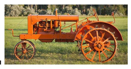
ordered as "air front," meaning rubber tires in front and steel wheels in back.
