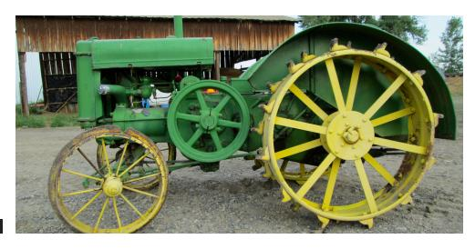
deal included Waterloo's experimental tractor designs and its sturdy 2-cylinder overhead-valve engine. John Deere continued the tractor development process and released the tractor as the Model D in 1923. Weighing just over two tons and costing around \$1,000, the Model D soon became a farm favorite.
