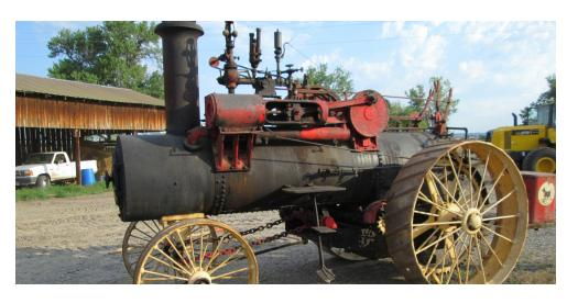
In 1887, Russell offered the 6 horsepower, which was equipped with self-adjusting piston rings, which freed up the task of lubrication. In the same year, Russell & Co. also create a 10-horsepower model, which included the patented features of a friction clutch, reverse gear, equilibrium valve, and boiler. In 1891, The 10-horsepower model, along with their 13-horsepower and 16-horsepower models, included a throttle lever, brake lever, steam chest, and reverse lever.
