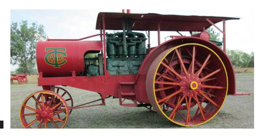
The Twin City 40-65 was the first in an impressive line of heavyweight gas tractors known as Twin City. Other models in the Twin City line included the 15-30, 25-45, 40-65, and a 14-ton, 6cylinder 60-90. The engine wasn't the only big feature of the 40-65. It weighed in at 12 tons and the rear wheels stood 84 inches high with 24" faces.
