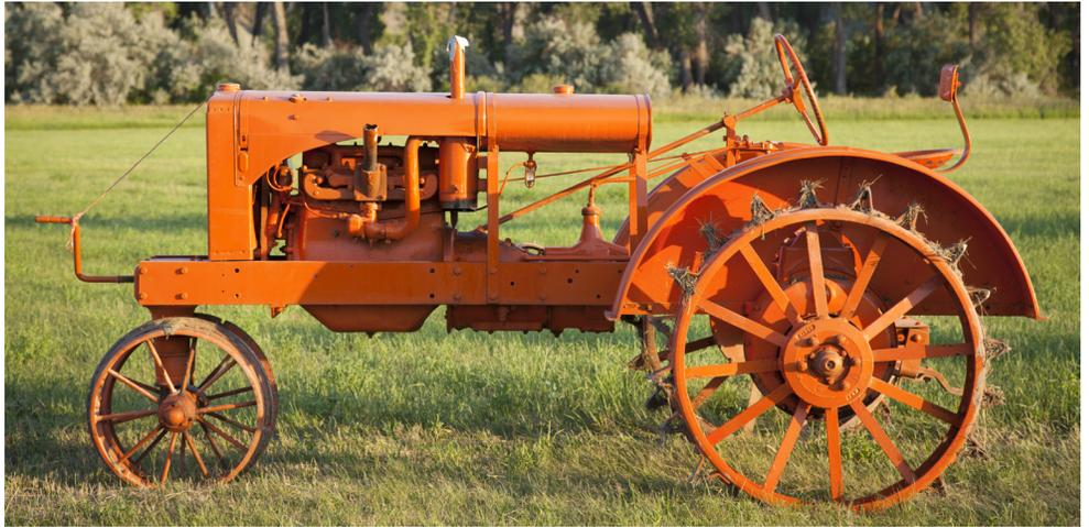
The Allis Chalmers Model WC was built from 1933 to 1948. The WC was designed from its start to be a nimble, low-cost, but well-powered row-crop tractor that would make the best use of pneumatic rubber tires, which Allis Chalmers had just introduced to agriculture in 1932. A very successful model, the WC was the best-selling tractor Allis Chalmers ever built.
