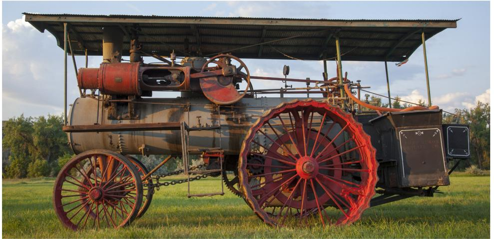
The Port Huron Engine and Thresher Co. began making steam rollers starting about 1890. They made a total of over 6,000 steam-traction engines along with portable steam, water wagons, threshers, sawmills, hay press balers, corn shellers, and other road-building machinery.
