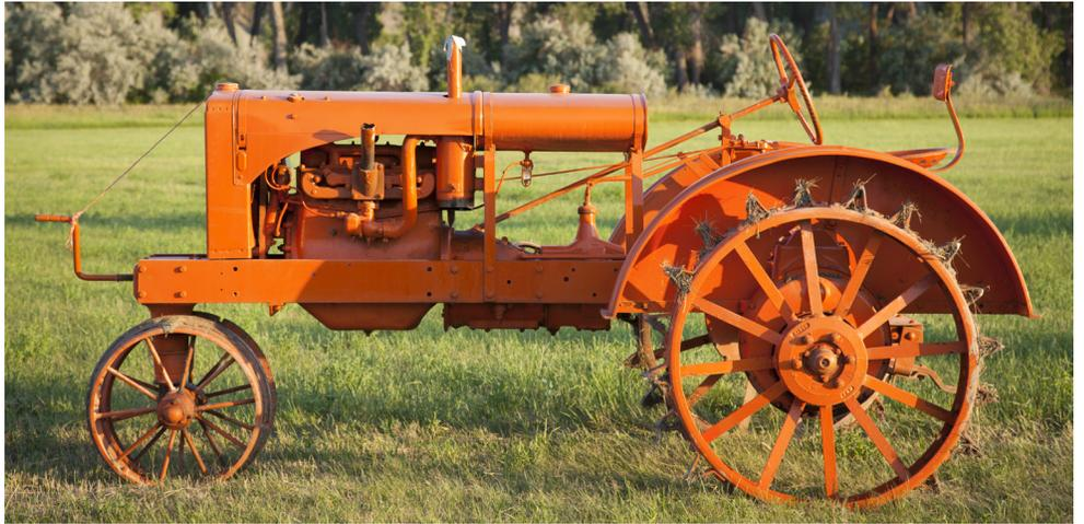
The Allis Chalmers Model WC was built from 1933 to 1948. The WC was designed from its start to be a nimble, low-cost, but well-powered row-crop tractor that would make the best use of pneumatic rubber tires, which Allis Chalmers had just introduced to agriculture in 1932. A very successful model, the WC was the best-selling tractor Allis Chalmers ever built.
